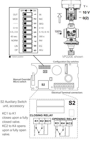
50VA transformer required per actuator.
