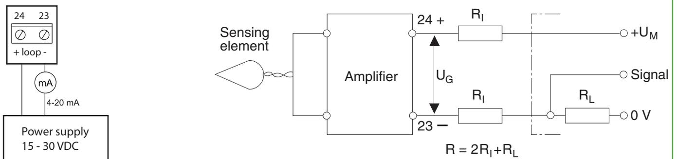
The transmitter is connected by a 2-wire cable, which serves for both the power supply and the signal transmission. Reading the measured signal value is achieved by having an external load resistance  $R_L$ .
