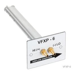
The VFXP Series probe is a differential air pressure device designed to measure air velocities in a duct. It includes multiple sensing points to measure total and static pressures. The VFXP Series incorprates a unique design to amplify the differential pressure by approximately 2.5 times for accurate measurement of lower air velocities down to 200 fpm. It is easy to install and cost effective.
